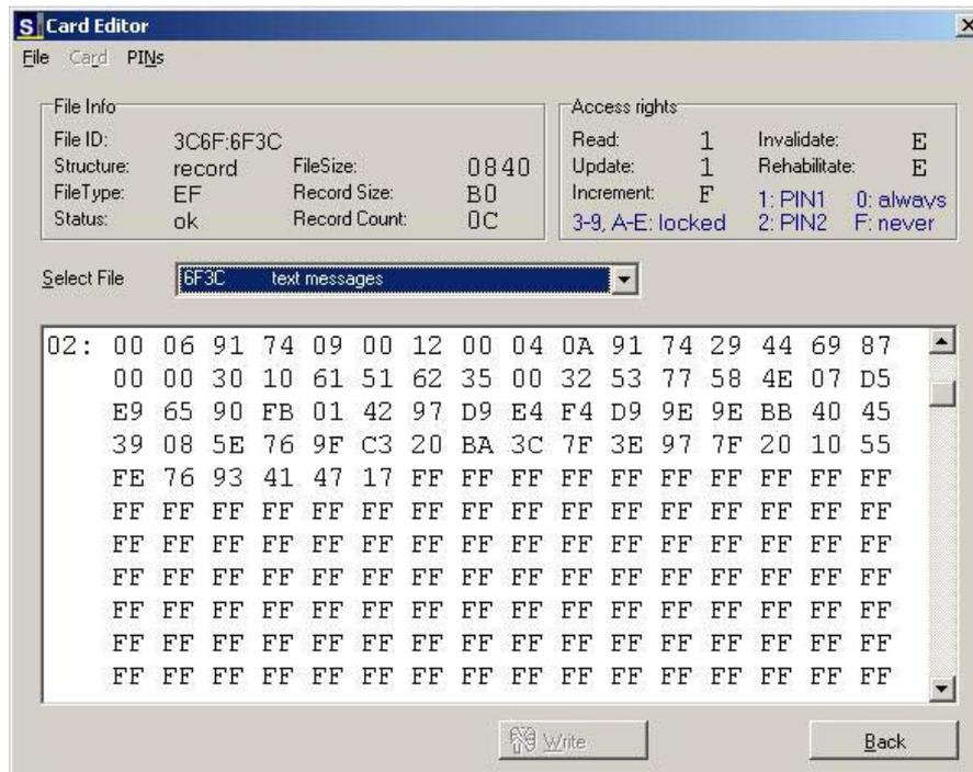
**Fig 3 – Reading a file as hex values with Sim-Surf Profi**
