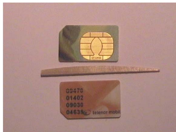
**Fig 2 – Subscriber Identity Module (SIM)**
