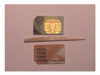
Fig 2 – Subscriber Identity Module (SIM)
